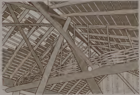
Wood framing supporting straw bales
