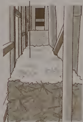
Wood framing supporting straw bales
